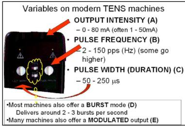
The machine will deliver 'pulses' of electrical energy, and the rate of delivery of these pulses (the *pulse rate* (B) will normally be variable from about 1 or 2 pulses per second (pps) up to 200 or 250 pps. To be clinically effective, it is suggested that the TENS machine should cover a rate from about 2 - 150Hz.
