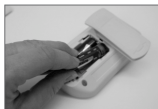
Figure 3-3 Insertion des batteries
